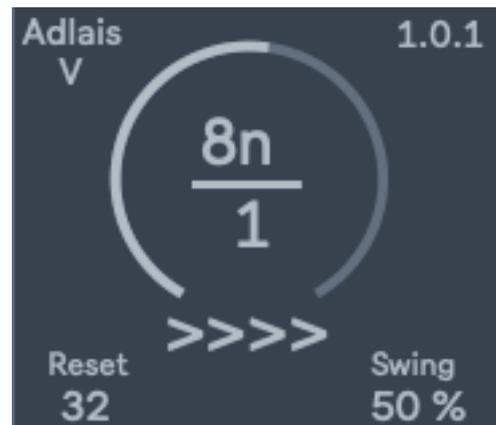
The number at the bottom of the fraction refers to a clock divider:
